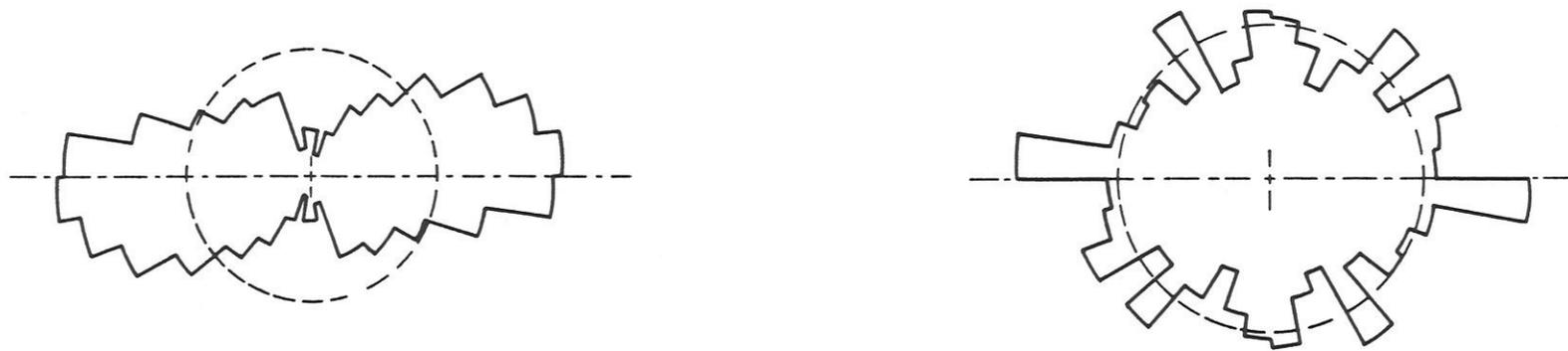
FIG. 2.4 Particle orientation diagrams on vertical sections of crushed basalt before and after dynamic compaction (52,53).
